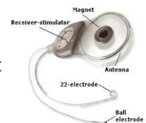
Figure 1. The internal component of the cochlear implant
